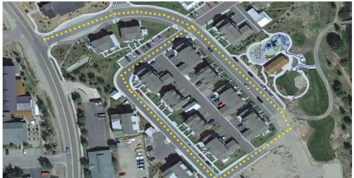
Aerial view of "TOD" development on the north of town adjacent to Airport Rd. Direct paths to access transit for pedestrians are not provided resulting in a longer walking distance to access transit.
